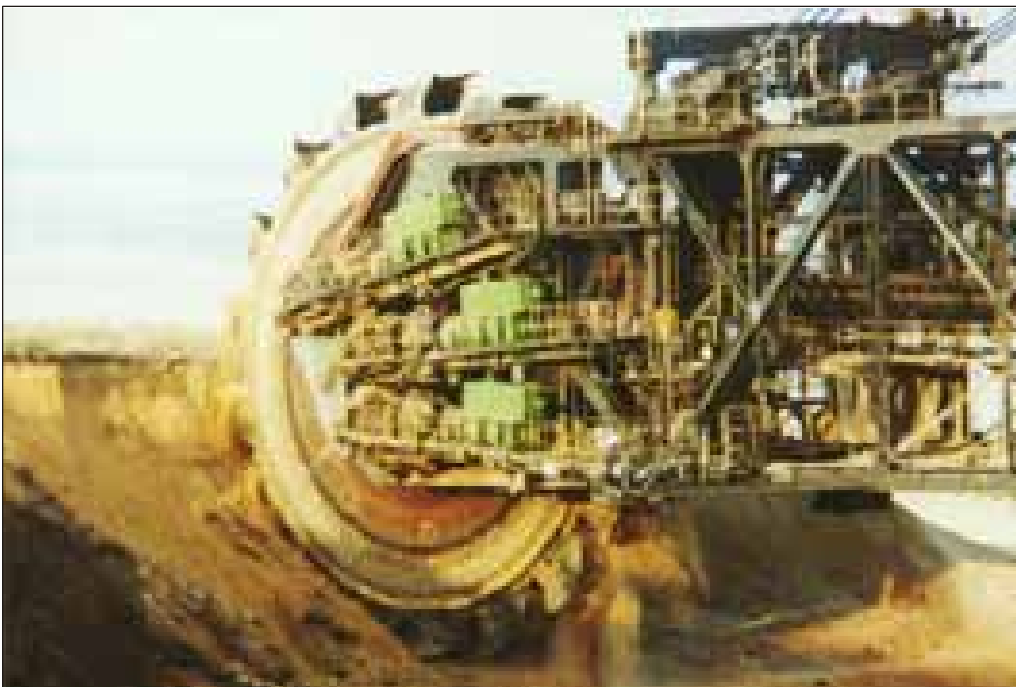
Laubag open-cast mine at Nochten, bucket wheel drive SRs 6300 equipped with 3 ELHY units, version EB 320/100 c320 SZm
